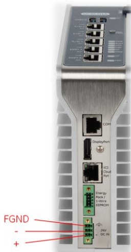
Figure 3: 24 VDC Power Input Connector
