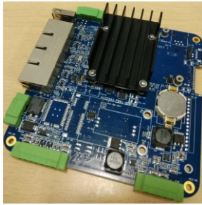
Figure 15: Supercapacitor Carrier Board
