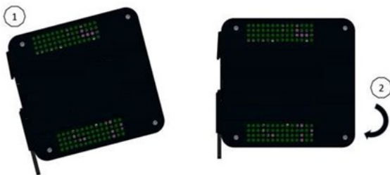
Figure 6: Mounting of the CPE115 on DIN rail
