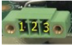
Figure 107: Power Socket (DN-IN1)
