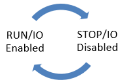
Figure 27: State Diagram for CPE100/CPE115 Run/Stop Operation
