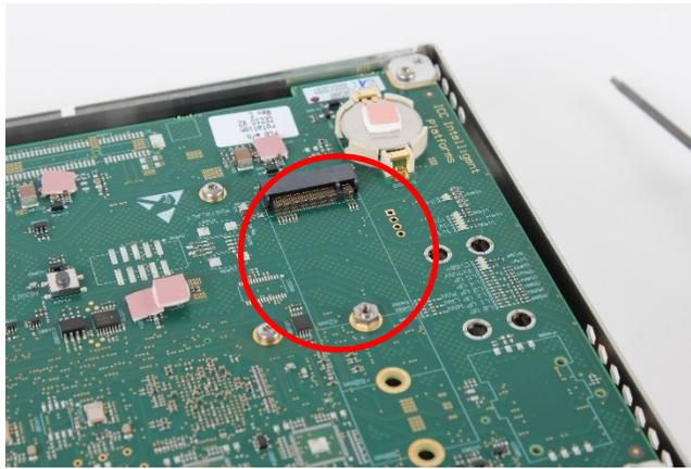
5. To insert a new M.2 storage device, connect the M.2 storage device in the slot and tighten the mounting screw to 0.45 Nm
