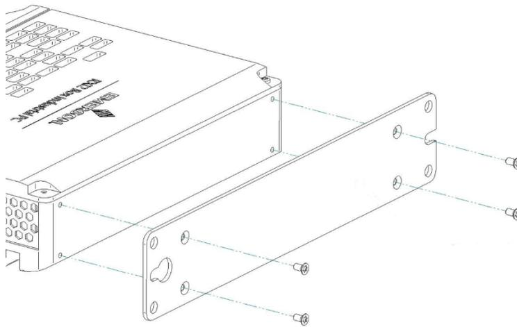
**Figure 5: RXi2-BP IPC DIN Rail pre-mounting**
