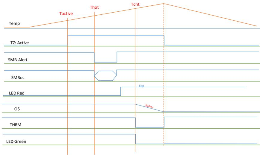
Note: Thermal Zone ‘Active’ is optional and not implemented in the RXi2-BP fanless design.
