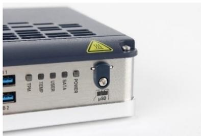
5. To remove the  $\mu$ SD card, remove the lid first and push it carefully in the same direction as step 3, the  $\mu$ SD card will pop out slightly and can then be removed.
