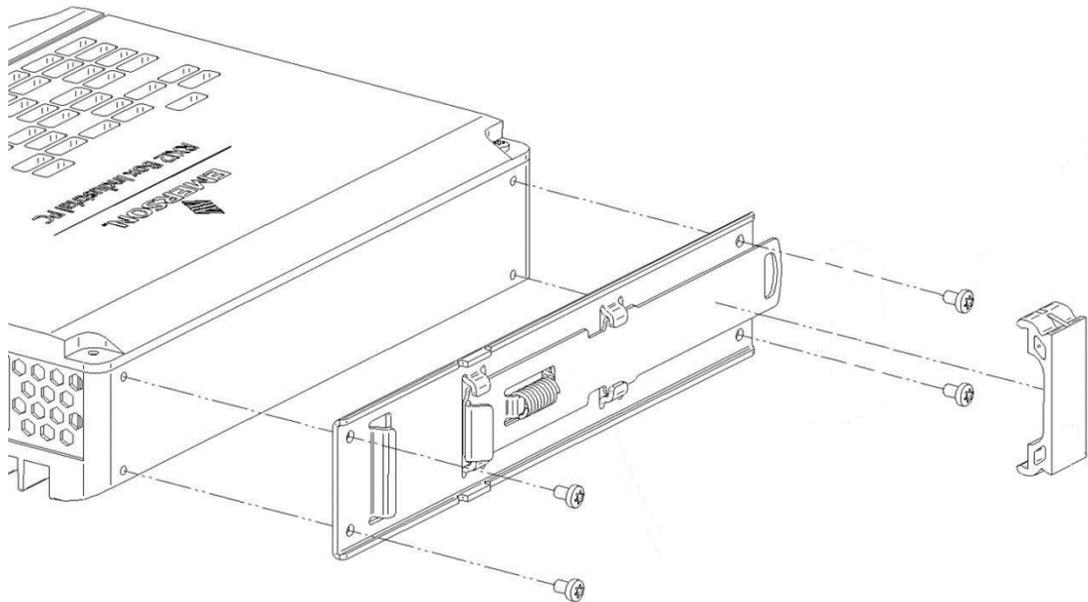
There are two DIN rail mounting options available, depending on the size of the DIN rail connector.
