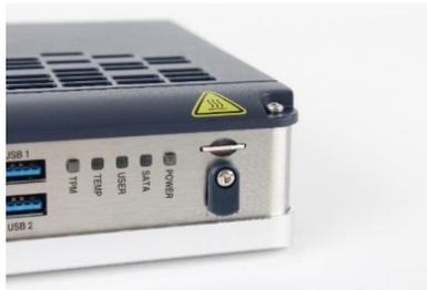
4. Re-attach the lid and tighten the screw to 0.45 Nm (Figure 12).
