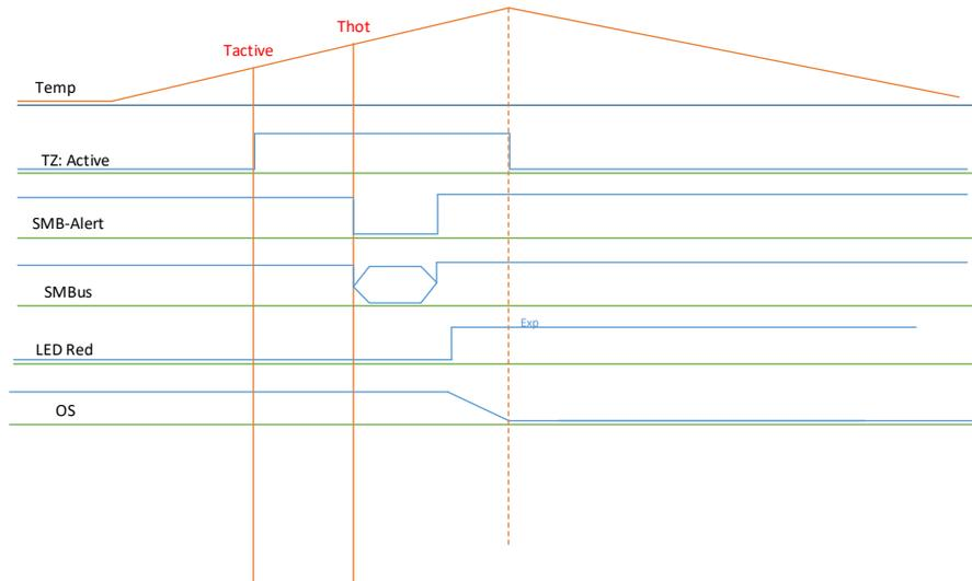
Note: Thermal Zone 'Active' is optional and not implemented in fanless RXi2-BP design.
