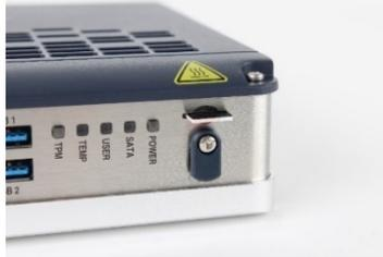
3. Plug-in  $\mu$ SD card until you hear a click. The populated connector is a push-push connector (Figure 11).
