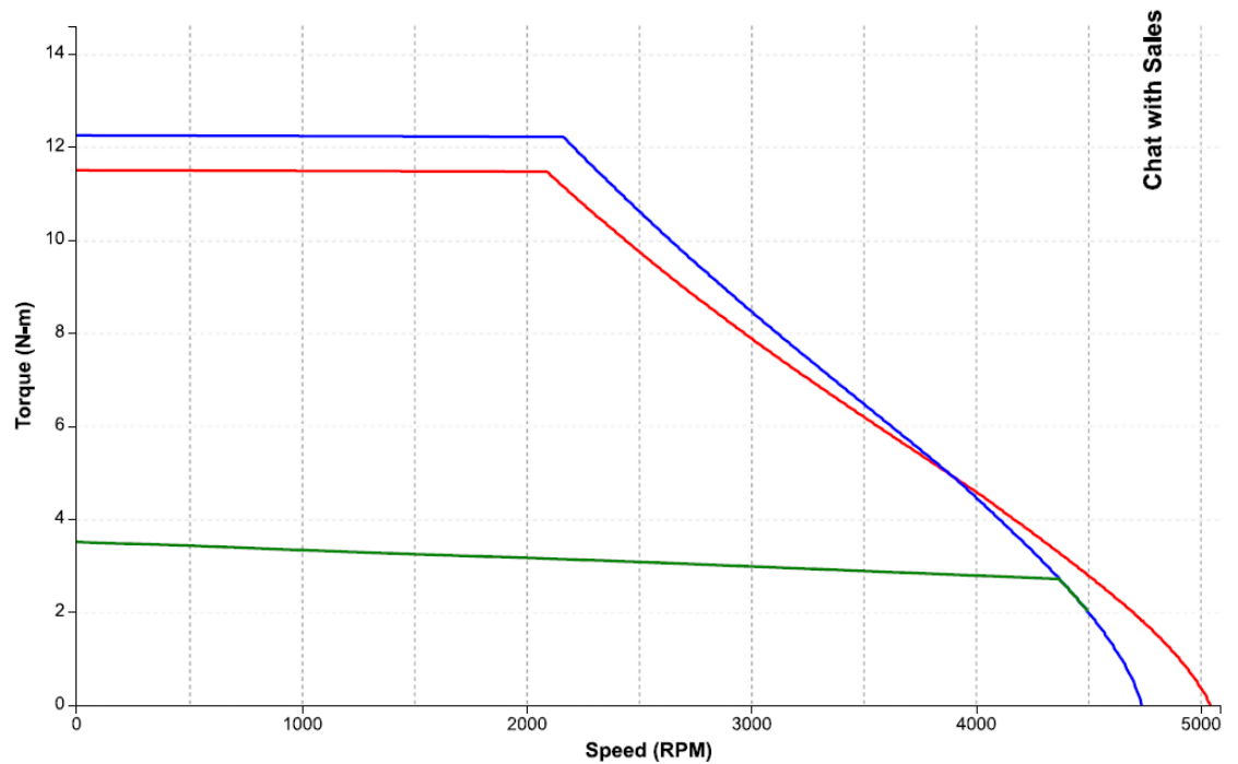
Figure 39: Speed-torque performance of an IC830M42G motor with an IC830DP01206 drive at 240 VAC
