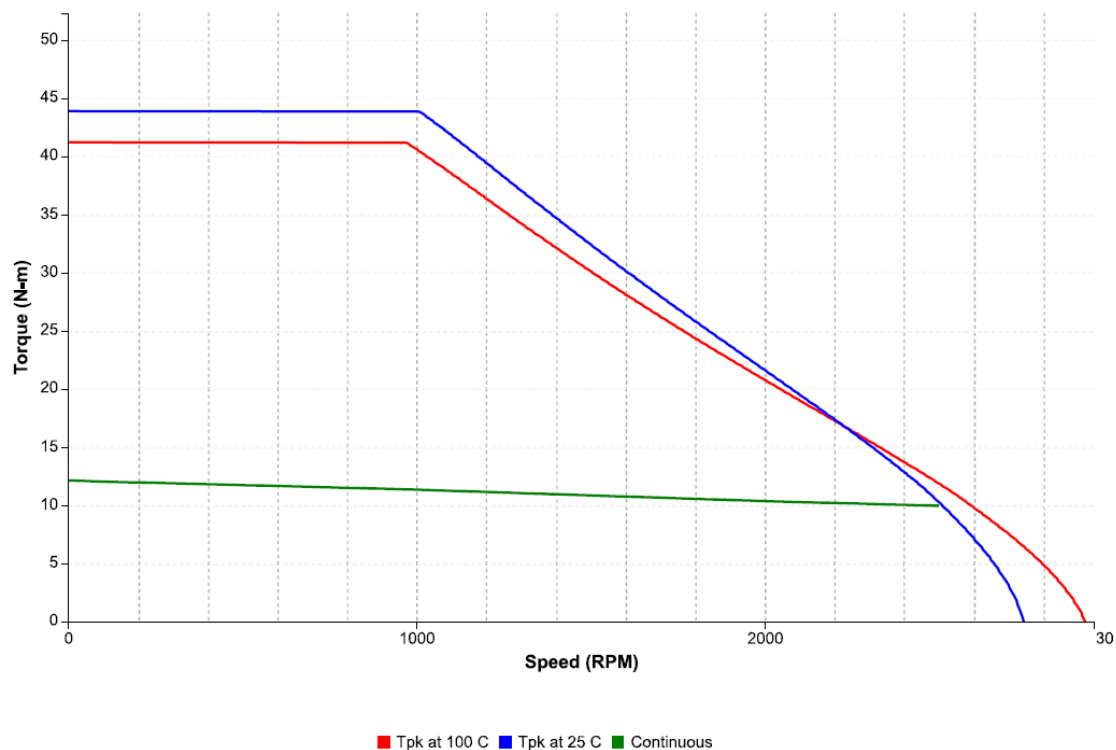
Figure 50: Speed-torque performance of an IC830M62H motor with an IC830DP02406 drive at 230 VAC
