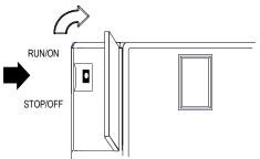
If the Run/Stop mode switch operation is enabled, the switch can be used to place the CPU in Run mode.
