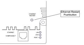
The Ethernet Restart pushbutton has two functions:
