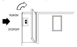
If Run/Stop mode switch operation is enabled, the switch can be used to place the CPU in Run mode.
