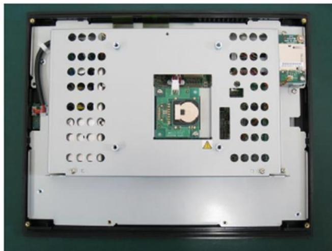
4. Gently remove the coin battery and replace with a new one, noting the polarity of the battery.
