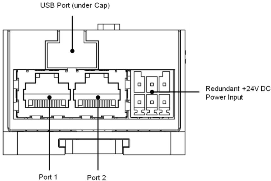
The two external RJ-45 Ethernet ports, which provide 10/100 Mbps copper interfaces, are on the bottom of the CEP001 Carrier.
