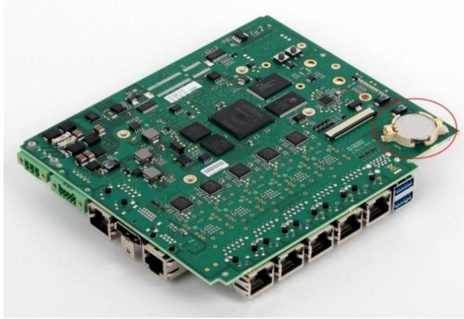
The CPE400/CPL410 is shipped with a real-time clock (RTC) battery installed on an internal circuit board (Figure 6). This battery will need to be replaced periodically by a qualified service technician. Typically, no action is required during initial installation.
