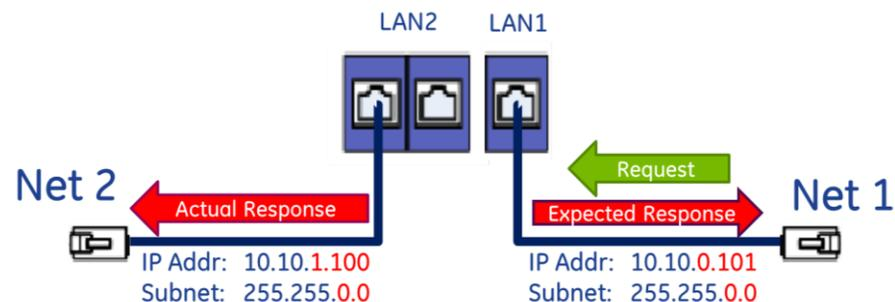
The issue demonstrated in Figure 47 is that requests entering one CPE330 interface can be routed out the other interface since both CPE330 Ethernet ports have been configured to be on the same network (255.255.0.0) but are physically connected to separate networks. Avoid this by assigning non-overlapping Subnets.
