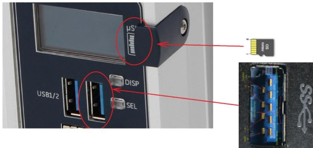
**Note:** The  $\mu$ SD-Card needs to be inserted in the slot with the correct orientation. The pins of the card need to face towards the front of the equipment (Figure 5). A cover and screw are provided. To minimize CPE400 susceptibility to electrical noise interference, keep the cover in place during normal operation.
