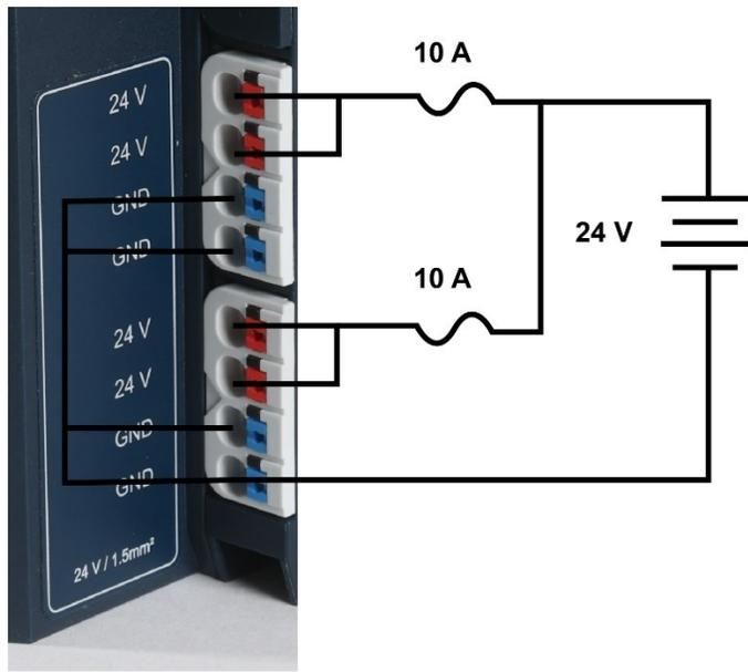
**Figure 33: Power Feed Maximum Current Draw**
