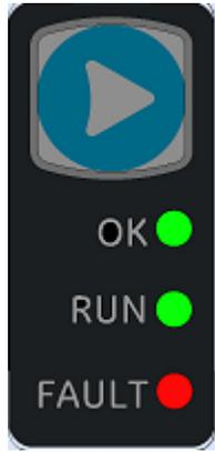
If the blue membrane pushbutton (Figure 25) is pressed while the CPE100/CPE115 is powering up, it restores the default IP address (192.168.0.100). It also erases the stored hardware configuration, logic, and contents of the backup RAM.
