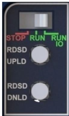
The RDS D and RUN/STOP Switches are located behind the protective door, as shown in Figure 10.
