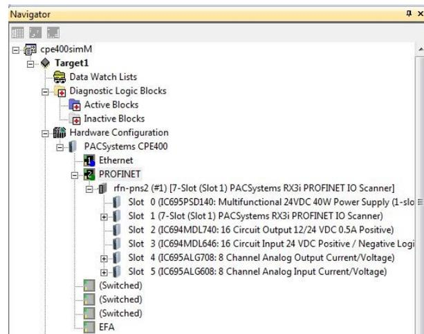
A PROFINET configuration may be transferred between a PROFINET Controller module (IC695PNC001) and the target Embedded PROFINET IO-Controller using the *cut/copy/paste* or equivalent drag and drop functions in PAC Machine Edition.
