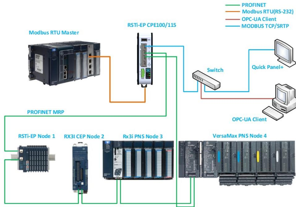
Whenever CPE100/CPE115 is configured for MRP only Ethernet Port2 & Port3 of LAN2 can be used to form a ring. Ethernet Port4 of LAN2 can still be used either to connect programmer, simplex PROFINET device or any other supported Ethernet protocols.
