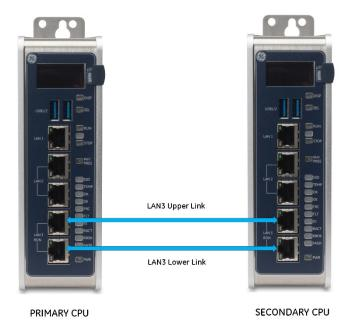
Note that CPE400/CPL410 LAN3 is used as a dedicated link, solely for CPU data synchronization in Hot Standby Redundancy Systems. Although the underlying network is a standard Ethernet network, no other Ethernet devices are permitted, except the two
