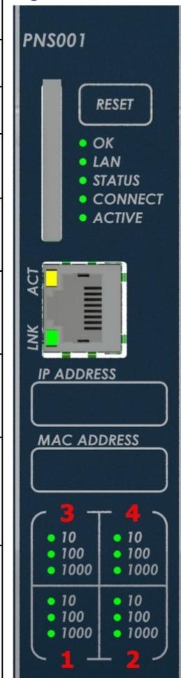
**Note:** Under certain ambient operating temperatures, the PROFINET Scanner could momentarily display the over-temperature pattern during power-up, while it is calibrating its thermal protection functions. This indication can be ignored. For details, refer to the section entitled *Microprocessor Over-Temperature* in *PACSystems RX3i PROFINET Scanner Manual*, GFK-2737.
