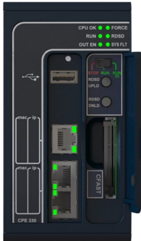
Figure 47: CPE330 (example of 2-Slot CPU)
