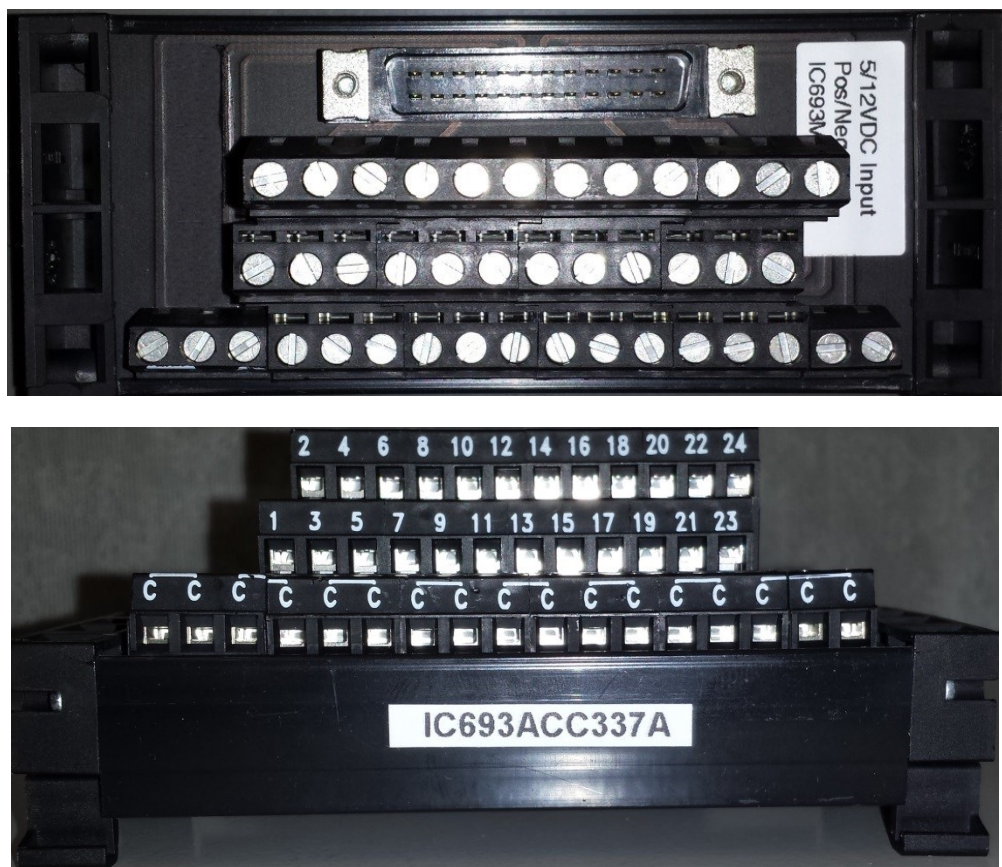
Figure 446: IC693ACC337 Terminal Block Top and Front Views
