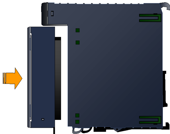
Figure 431: Installing a High-Density Terminal Block
