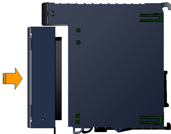
Figure 431: Installing a High-Density Terminal Block
