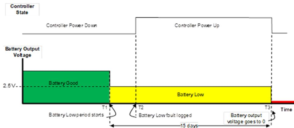
The Battery Low period of 15 days starts at Point T1, but the low battery fault is logged at Point T2, when the controller is powered ON. The user should be aware that the Low Battery fault timestamp does not indicate the start of the 15-day Battery Low period.
