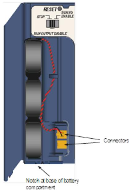
Figure 6: RX7i Battery Installation
