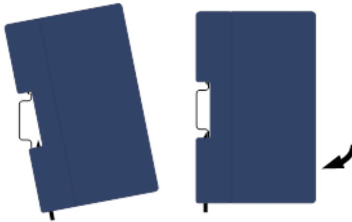
**Note:** To remove the Energy Pack from the DIN rail, use a small flat-blade screwdriver to pull down on the tab on the bottom of the Energy Pack and then lift the module off the DIN rail.
