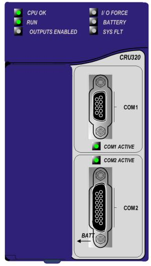
The PACSystems\* RX3i Redundancy CPU can be used to perform real time control of machines, processes, and material handling systems. The CPU communicates with the programmer and HMI devices via a serial port using SNP Slave protocol. It communicates with I/O and smart option modules over a dual backplane bus that provides:
