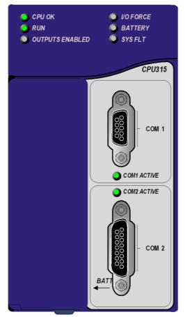
The PACSystems\* RX3i CPU can be used to perform real time control of machines, processes, and material handling systems. The CPU communicates with the programmer and HMI devices via a serial port using SNP Slave protocol. It communicates with I/O and smart option modules over a dual backplane bus that provides:
