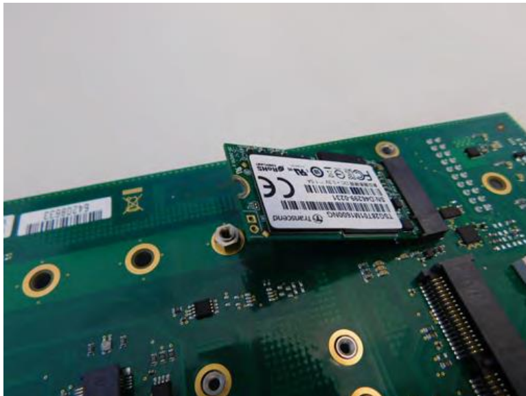
Figure 4-23 M.2 M-Key Insertion into Connector Slot
