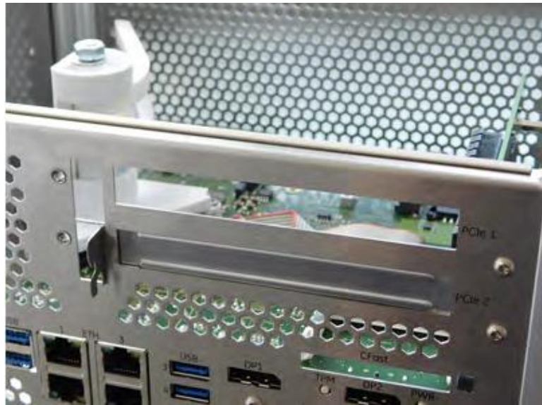
Figure 4-4 Removed PCIe Slot Bracket
