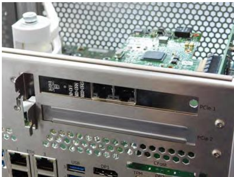
Figure 4-5 PCIe Board Bracket Inserted into Slot
