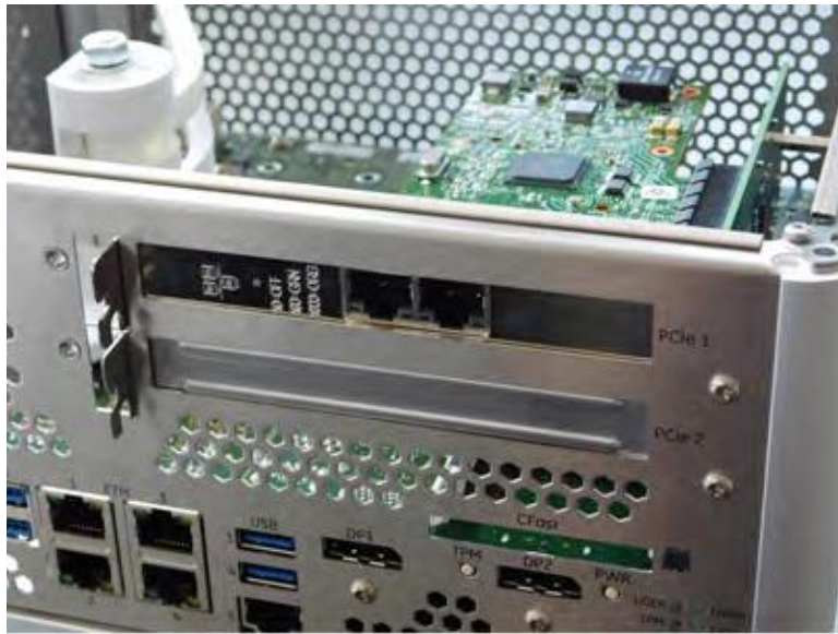
Figure 4-6 PCIe Board Bracket Inserted into PCIe Connector
