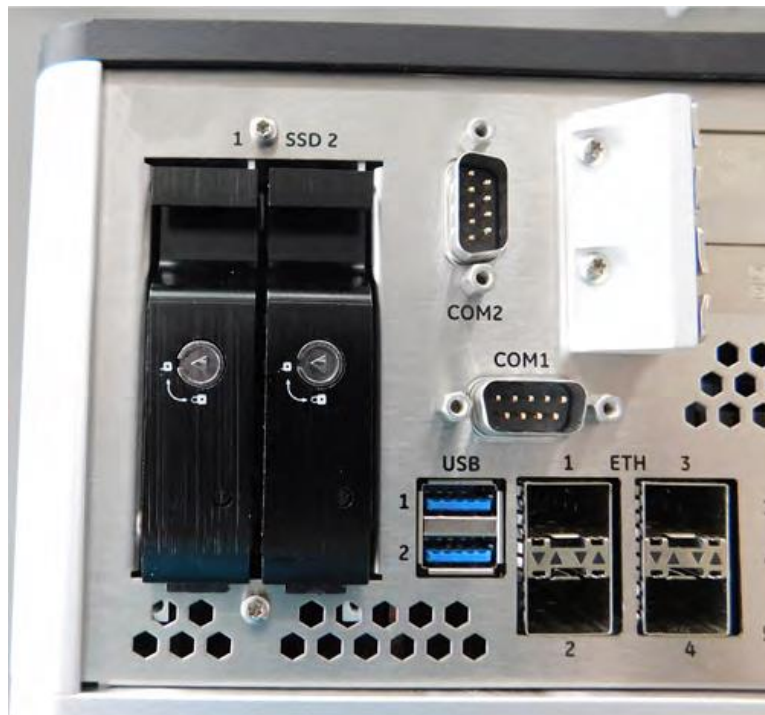
Figure 5-21 Insert the tray
