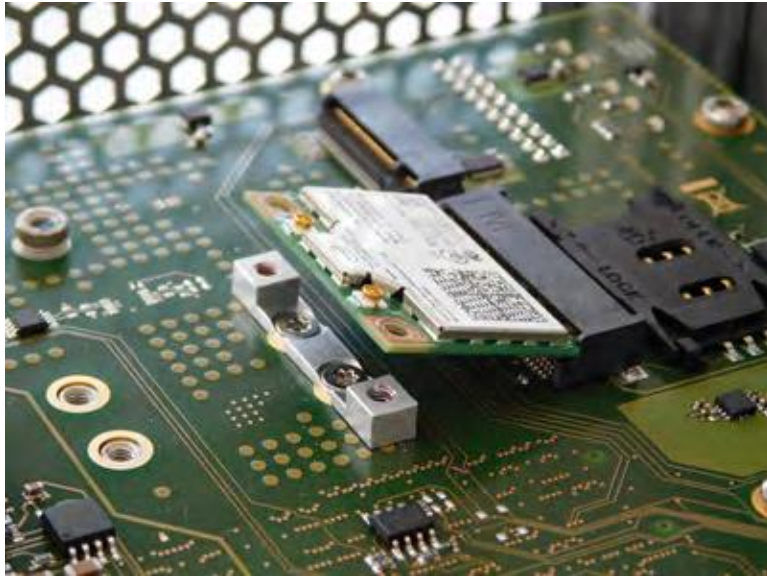
Figure 4-13 Mini PCIe Board Inserted
