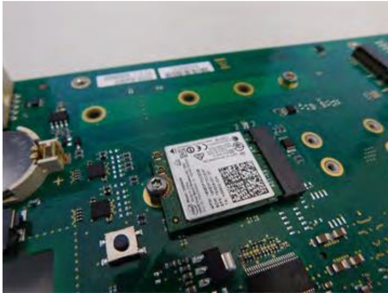
Figure 4-21 M.2 A-Key Mounted to RXi2-EP IPC
