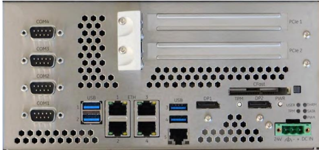
Figure 5-2 RXi2-EP IPC Hardware Interface Overview (2-slot Option)
