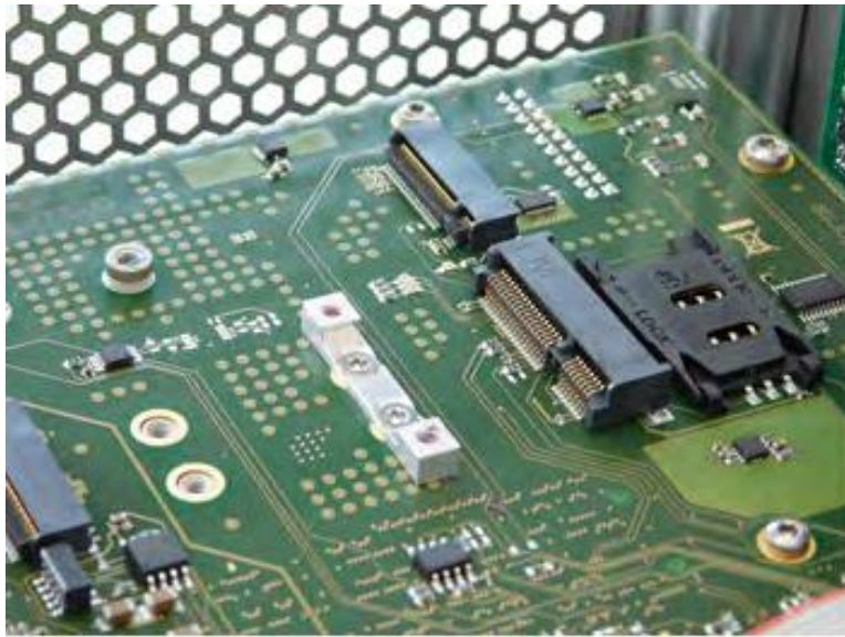
Figure 4-11 Short Position for mPCle Bracket
