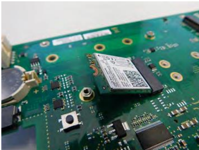
Figure 4-20 M.2 A-Key Insertion into Connector Slot
