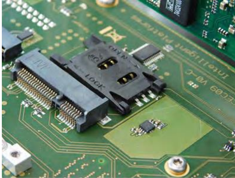
Figure 4-15 SIM Interface Connected to mPCIe – Unlocked but Closed
