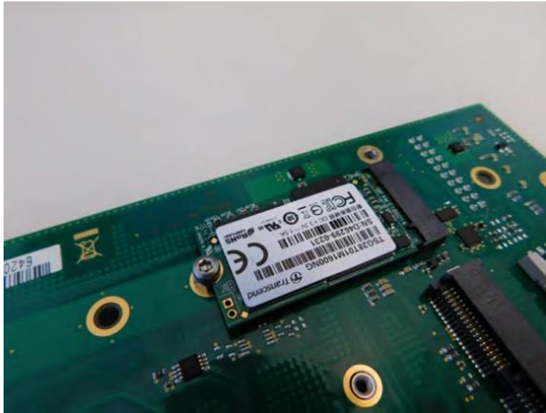
Figure 4-24 M.2 M-Key Mounted to RXi2-EP IPC
