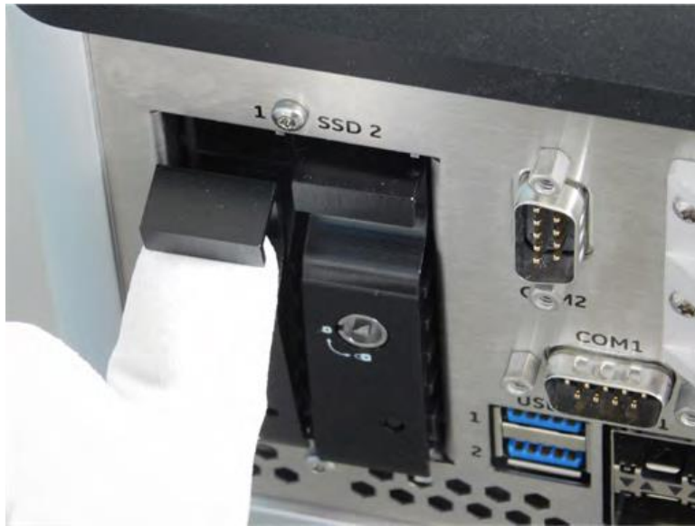
Figure 5-15 Removing Storage Device Tray from Mounted Position
