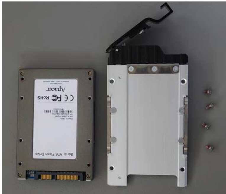
Figure 5-19 Insert the replacement hard drive
