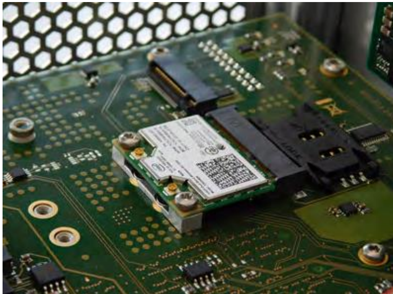
Figure 4-14 Mini PCIe Board Mounted to RXi2-EP IPC
