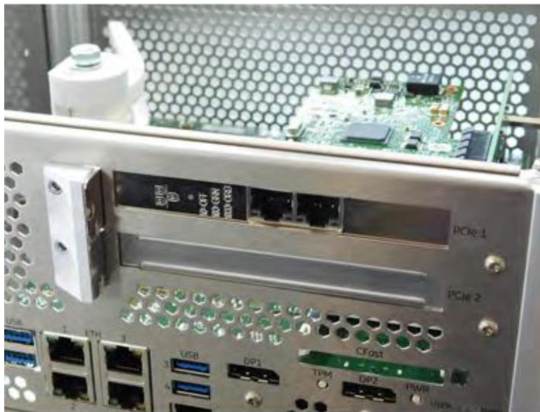
Figure 4-7 Reattached PCIe Support Bracket
