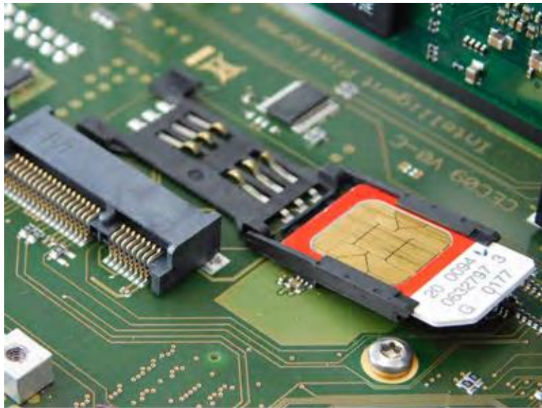
Figure 4-17 Inserted SIM card
