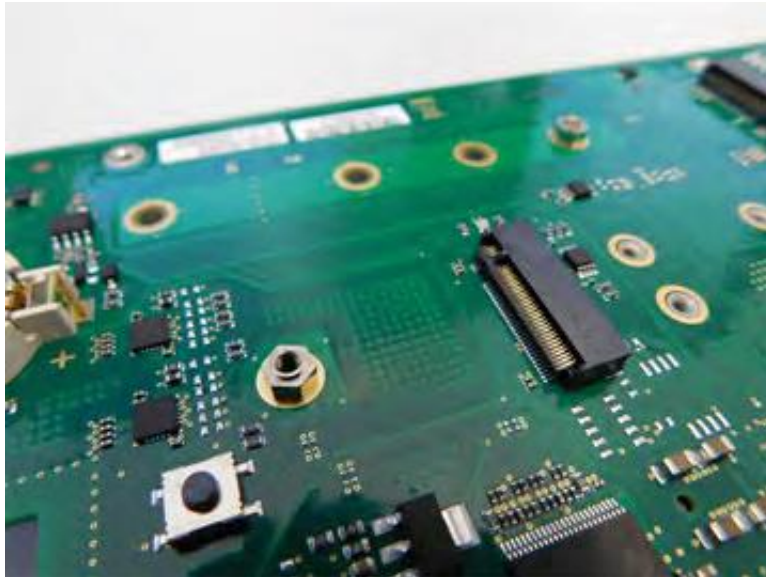
Figure 4-20 M.2 A-Key Insertion into Connector Slot
