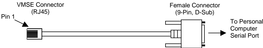
Figure 6-8. Cable for Serial Monitor/Load of VMSE
