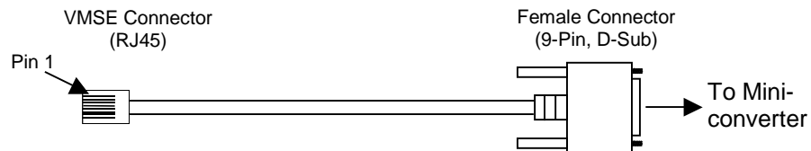
Figure 6-6. VMSE RJ45 Serial to RS232/485 Miniconverter
