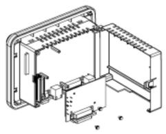
Disconnect the DC input power terminal block connector from your QuickPanel Control unit before connecting the Communication Module to the unit.
