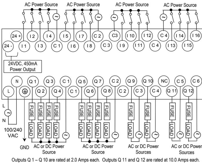
**NOTE: All DC inputs can be connected as either positive or negative logic. The example diagrams in this datasheet show positive logic connections.**
