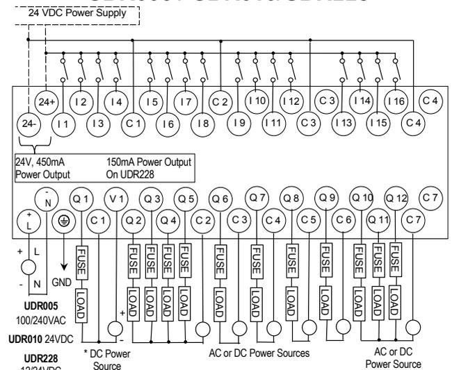
\* A pulldown resistor connected between Q1 and C1 is required for high frequency Pulse and PWM outputs and for duty cycles in the lower ranges (5% and lower). A 1.5k Ohm, 0.5 watt resistor is recommended.
