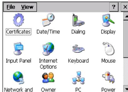
The certificate itself is imported with the Certificates control panel applet. The main requirements of the certificate are that it must have the server authentication key usage attribute set and the name of the certificate should match the name used to connect to the FTP server (which could be the IP address of the server).
