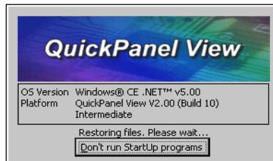
When the switch is set to “ON”, the startup programs are forced to run and the “Don’t run Startup Programs” button is not available on the startup splash screen.
