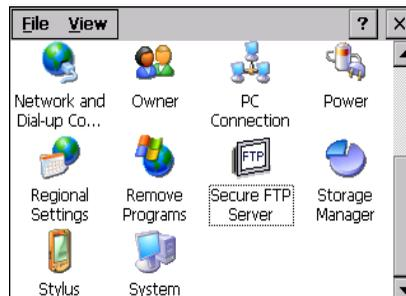
All configuration of the FTP server is accomplished with the Secure FTP Server control panel applet. By default, the server is not enabled. Once enabled, a background program will run, waiting for clients to connect. Up to ten
