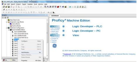
Once "added" to the rack location, set up the EDS001 parameters in the "Settings" and "RS-232 Port (Station Manager)" tabs as needed for the application.
