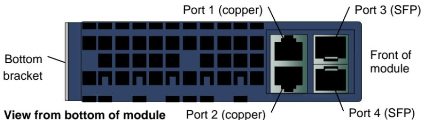
The module is assigned five Ethernet MAC addresses: one for each of the four external Ethernet ports and one for the internal switch.
