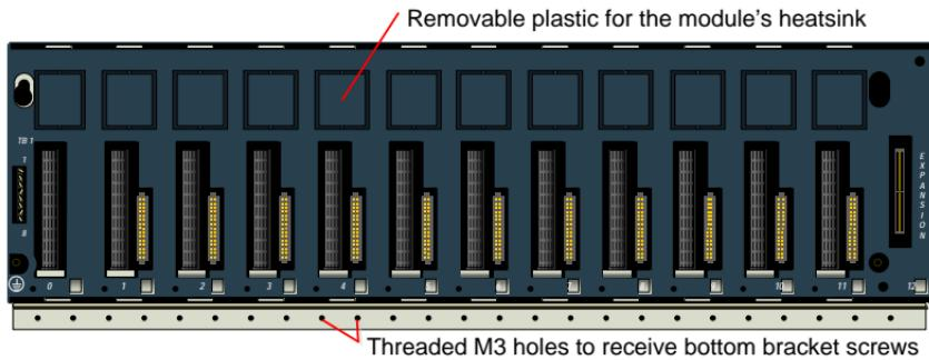
The installation slot must match the slot that is selected in the module's hardware configuration in the Proficy® Machine Edition application.
