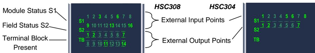
The Module Status (S1) LED indicates the status of the module. Solid green indicates that the module has been configured. Blinking green indicates no configuration. Blinking amber/yellow indicates a fatal module failure.
