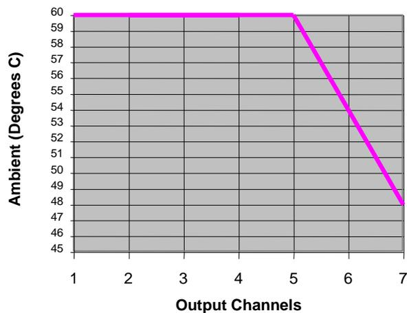
For module IC695HSC308, more output channels can be used at the same time at a given ambient temperature when outputs are evenly distributed into two groups. If outputs are either set up as one output group or unevenly distributed between two output groups, fewer output channels can be used for a given ambient temperature.
