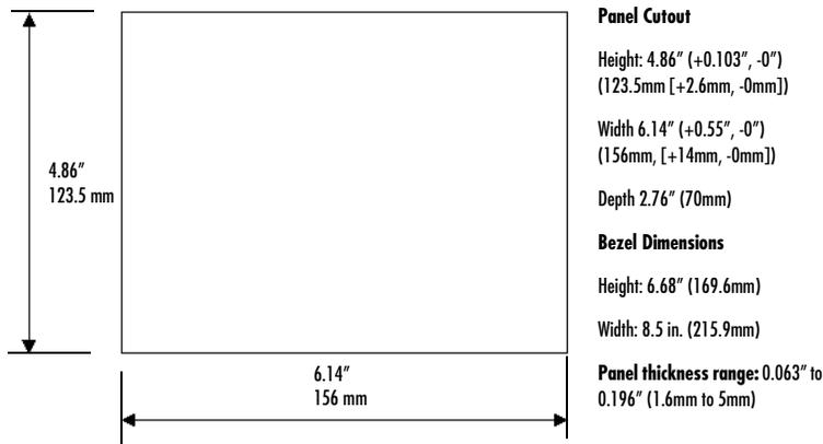
The unit will **not** fit through the small cutout with a CF card inserted in the port, with any cables connected, or with the power supply plug inserted in the socket.
