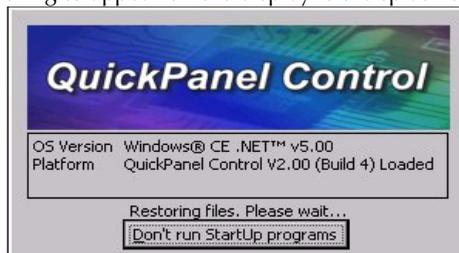
2. To skip running any programs included in the StartUp folder, tap **Don't run StartUp programs**. The splash screen disappears automatically after about 5 seconds. The Windows CE desktop then becomes visible.
