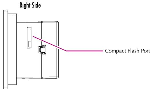
A CF card is inserted in this port with its front facing the front panel of the unit (the narrow side slot on the card should be toward the top). The card should slide in easily—to avoid damage, do not force it.
