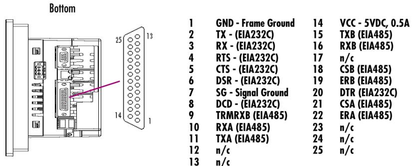
**Note:** Pin 14 is fused with a field-replaceable, 1.0A fast-blow fuse.
