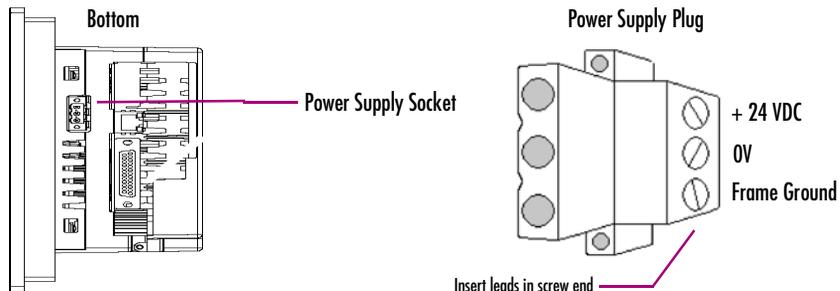
**Note:** The torque range for the attaching screws is 4-6 inch/lbs.
