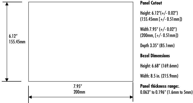
To secure the QuickPanel View/Control to a panel with the large cutout, use the four included mounting clips, which hook into the openings located on the top and bottom of the housing, as well as the four included clip extensions, which slide over the inner portion of the bezel as shown in the following illustration.
