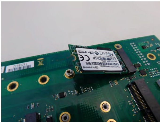
Figure 34: M.2 M-Key Mounted to RXi2-UP IPC
