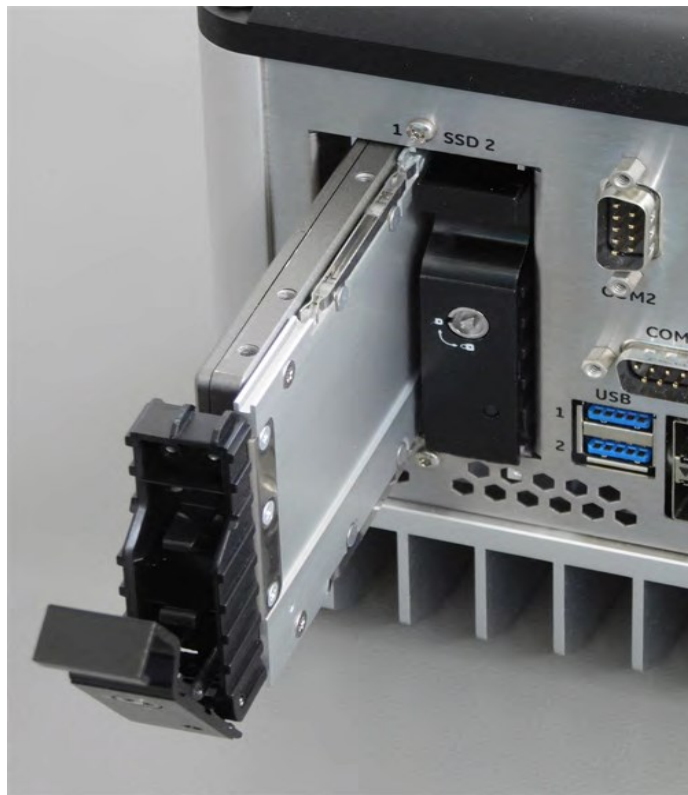
Figure 52: Removal of Storage Device Tray
