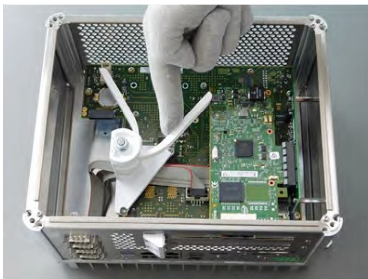
Figure 19: Card Holder Adjustment
