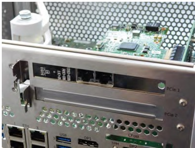
Figure 15: PCIe Board Bracket Inserted into Slot
