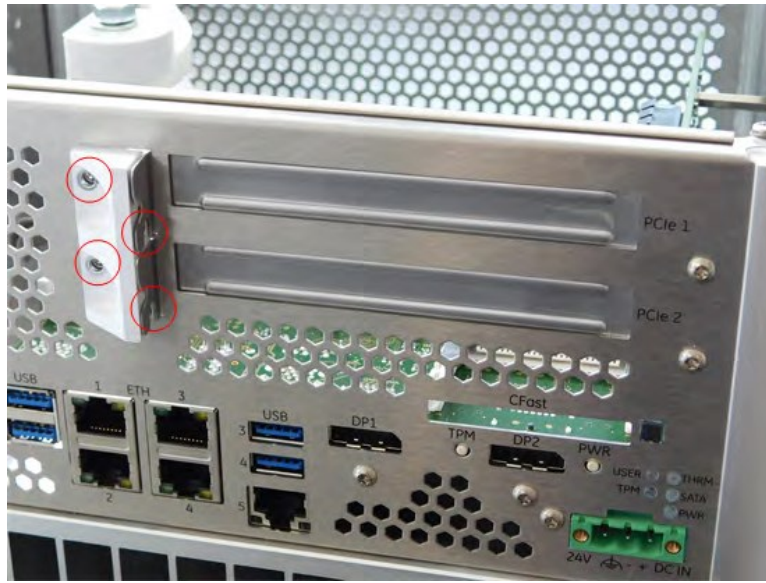
Figure 12: PCIe Support Bracket Screws
