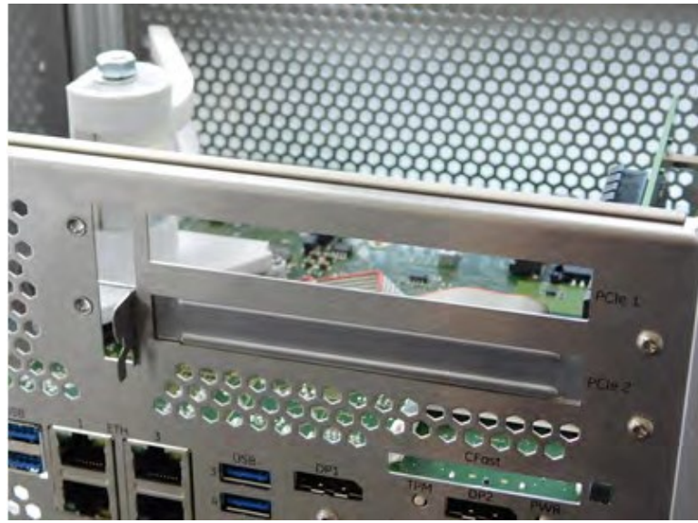
Figure 14: Removed PCIe Slot Bracket
