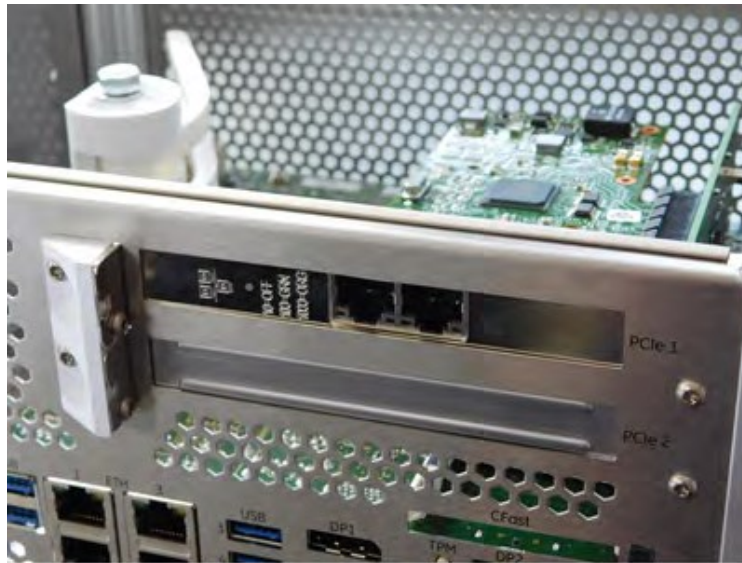
Figure 18: Reattached PCIe Bracket Screws
