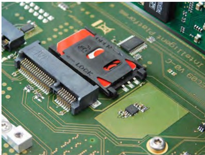
Figure 28: SIM Card Holder Closed and Locked
