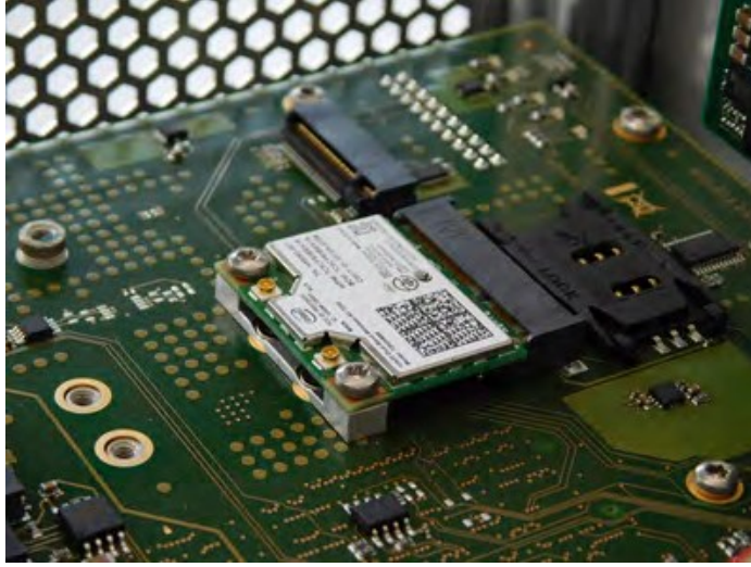
Figure 24: Mini PCIe Board Mounted to RXi2-UP IPC
