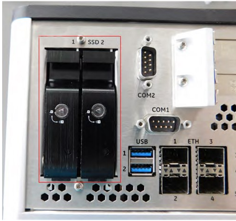
Figure 49: 2.5 inch SATA Drive Device Tray Location
