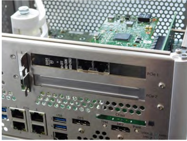
Figure 16: PCIe Board Bracket Inserted into PCIe Connector
