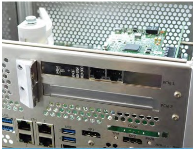
Figure 17: Reattached PCIe Support Bracket
