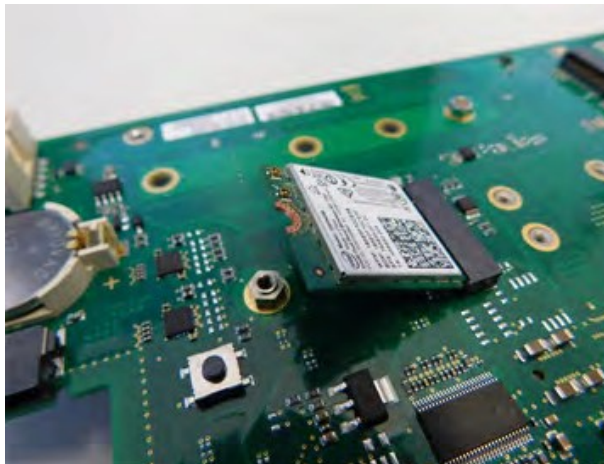
Figure 30: M.2 A-Key Insertion into Connector Slot
