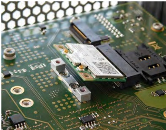
Figure 23: Mini PCIe Board Inserted
