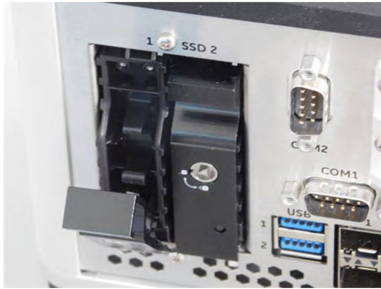
Figure 51: Storage Device Tray Fully Open Position
