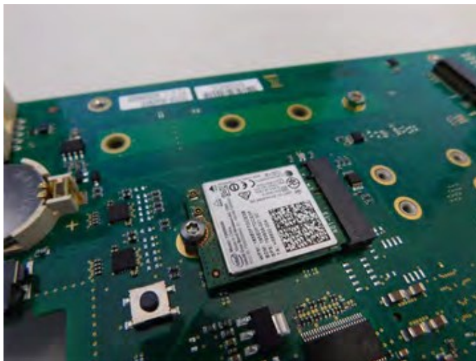
Figure 31: M.2 A-Key Mounted to RXi2-UP IPC
