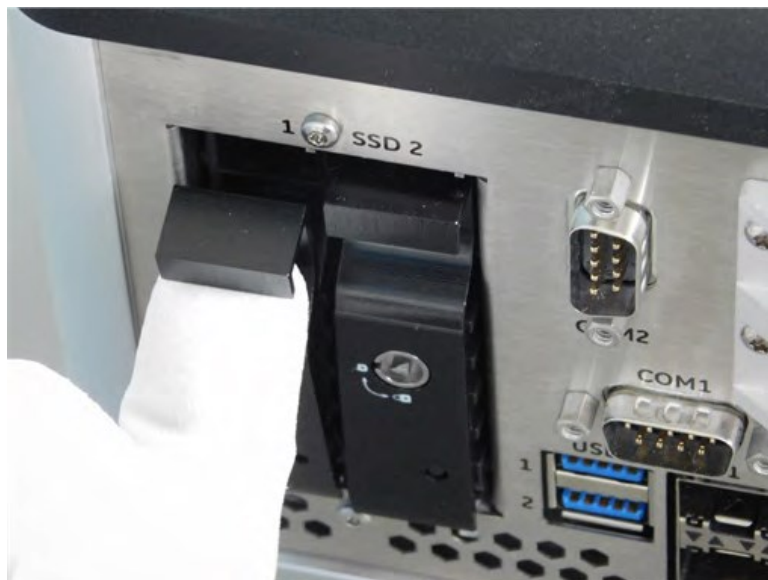
Figure 50: Removing Storage Device Tray from Mounted Position
