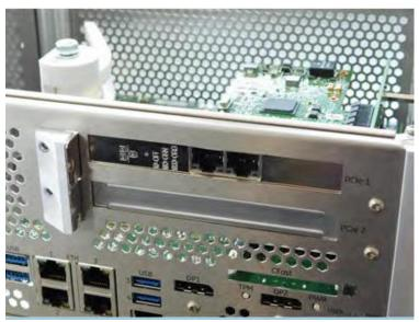
Figure 4-7 Reattached PCIe Support Bracket
