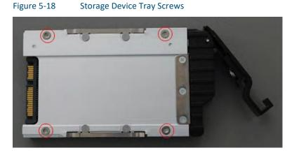
6. Insert the replacement hard drive and screw in the four mounting screws to mount it.
