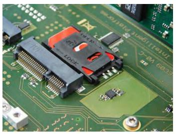
Figure 4-18 SIM Card Holder Closed and Locked
