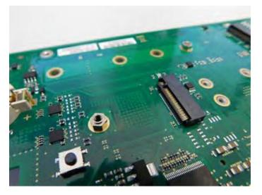
Figure 4-20 M.2 A-Key Insertion into Connector Slot
