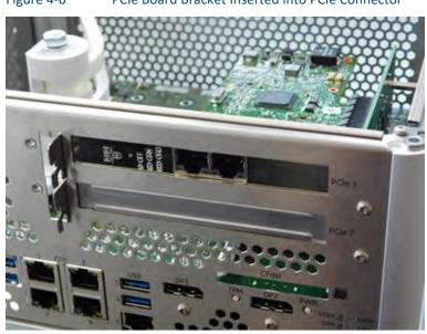
Figure 4-6 PCIe Board Bracket Inserted into PCIe Connector
