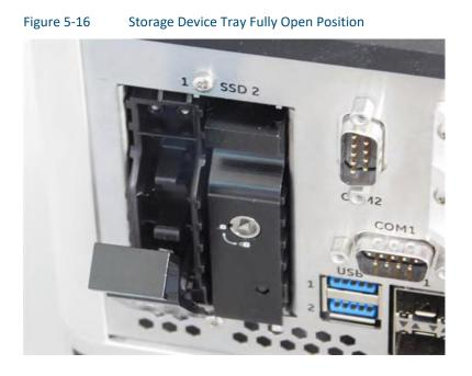
4. Remove the hard disk tray completely from the unit.
