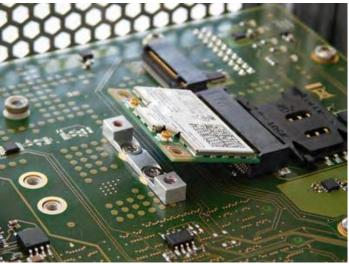
3. Mount Mini PCIe board into the connector slot using standard screws (Tx8 [0.6 Nm/5.3 in lb]) screw: ISO14583 M2.5 x 6 or M2.5 x 5.
