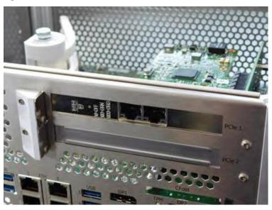
Figure 4-8 Reattached PCIe Bracket Screws
