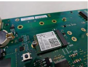
Figure 4-22 M RXi2-UP IPC Connector Slot
