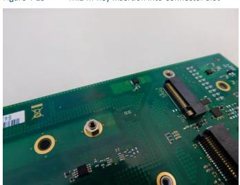
Figure 4-23 M.2 M-Key Insertion into Connector Slot
