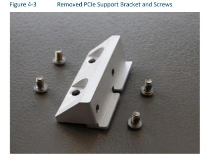
4. Remove the PCIe slot bracket.
