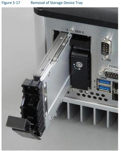
5. Unscrew the four mounting screws and separate the hard drive from the tray.
