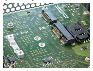
2. Insert the Mini PCIe board into the connector slot.
