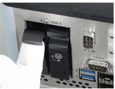
Figure 5-15 Removing Storage Device Tray from Mounted Position
