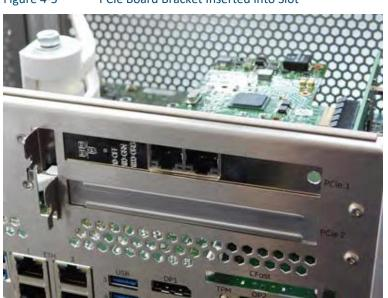
Figure 4-5 PCIe Board Bracket Inserted into Slot
