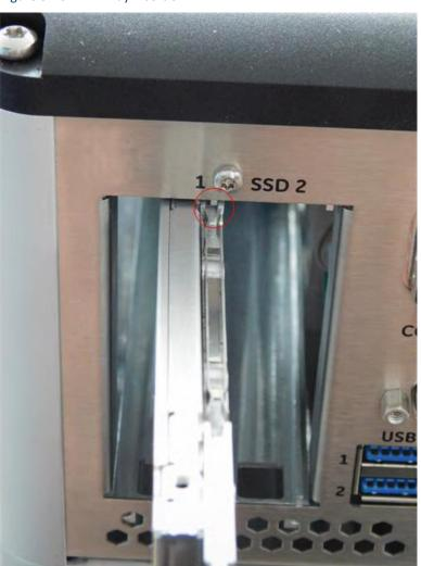
Figure 5-20 Tray insertion 8. Insert the tray until it is fully and firmly seated.
