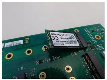
Figure 4-24 M.2 M-Key Mounted to RXi2-UP IPC
