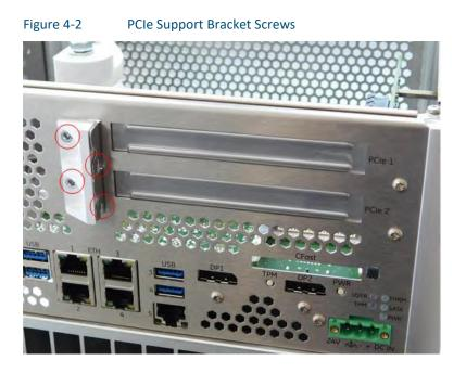
3. Remove the PCIe support bracket.
