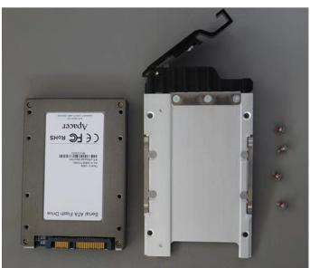
7. Insert the storage device tray ~25.4 mm (1 in) (maximum) into the slot, move it to the right side until the nose is between the guidance mark of the tray, then push it carefully into the slot.
