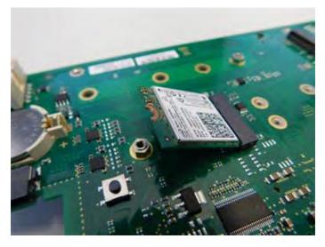
2. Mount the M.2 A-Key board into the connector slot using standard screws (Tx8 [0.45 Nm/5 in lb]), screw: ISO14583 M2.5 x 6, or M2.5 x 5.
