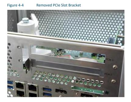
5. Insert the PCIe board bracket into the slot.
