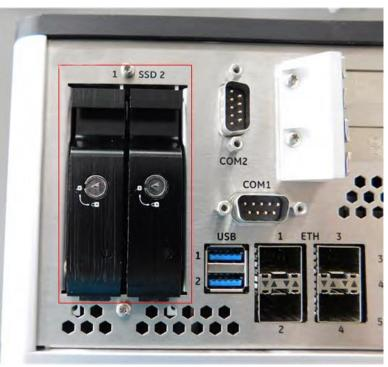
2. Insert your finger under the handle and carefully remove the storage device tray from the mounted position.
