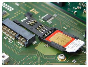
Lock the SIM card into position by moving the upper part in the LOCK ← direction (as shown on the part).
